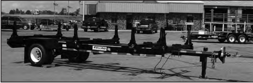
Shown to the left: Utility Pole Trailer with Tongue Retracted
