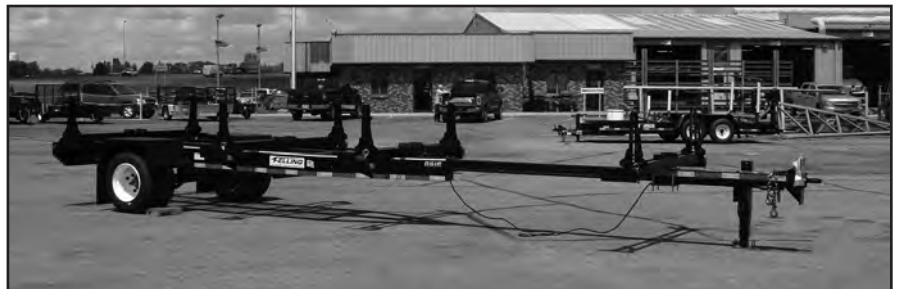
Shown above: Utility Pole Trailer with Tongue Extended
